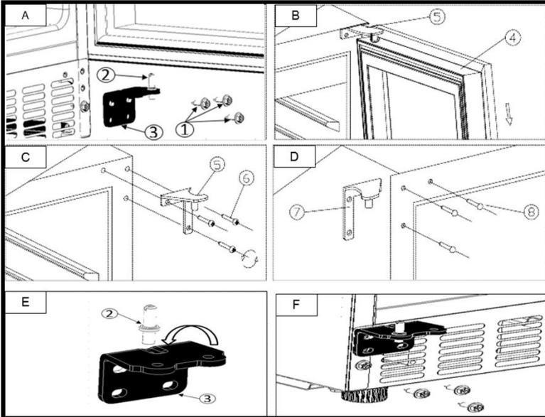
1 Screws 2 Hinge axis 3 Lower hinge 4 Door 5 Top hinge (Right) 6 Screws
